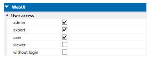
Select the checkbox to specify for each web user interface user profile whether the ASM is displayed on the web user interface. This setting does not have any effect on the rights for the related user profile in the detailed view for the ASM on the web user interface.
