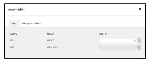
A field is displayed on the web user interface for each function element of type WEB IN and WEB OUT used in your logic. All users except the "Viewer" have access and can enter data.
