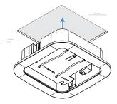
**6** Using a Phillips screwdriver, press each spring-loaded dogleg lever in, then 1/4 turn clockwise until the lever is perpendicular to the bracket edge, then release it. The spring-loaded doglegs hold the bracket securely in place.
