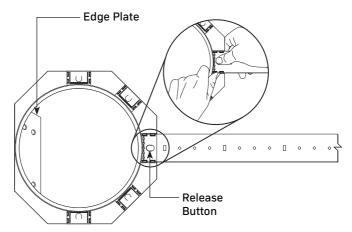
The in-ceiling speakers include an egde plate to secure if mounting the speaker against a joist.
