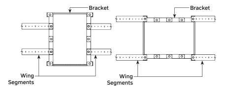
2. Use the 1" markers as a placement guide for aligning the brackets. Drive a screw through the metal wings to secure into the desired position.
