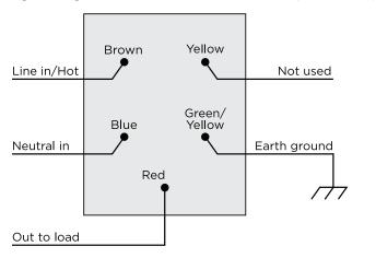
Figure 3. Single device location, without neutral connection
