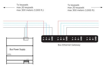
Daisy chain topology with gateway and two power supplies in the middle of the chain
