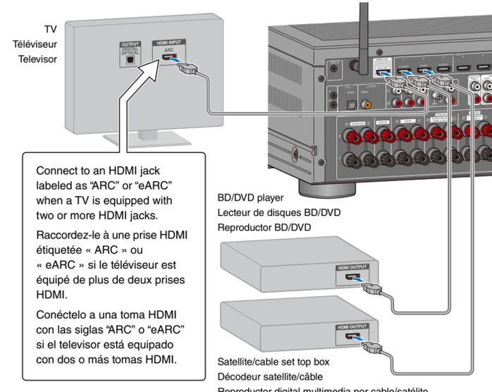
Connect to an HDMI jack labeled as "ARC" or "eARC" when a TV is equipped with two or more HDMI jacks.
