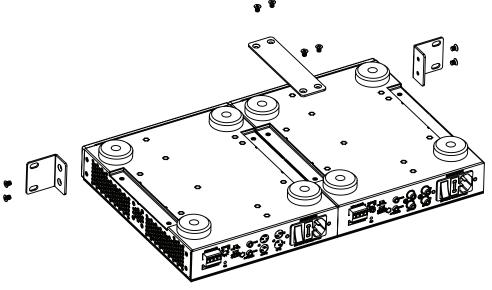
**Note:** Rack ears can be installed to the front or the back of the amplifier as needed.
