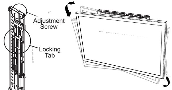
Figure 7 Pull out and away from the wall
