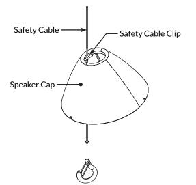
**6.** Thread the speaker cap onto the gripple and temporarily secure it with the safety cable clip on the cap.
