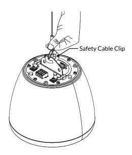
**8.** Connect the hook on the cable to the 3-hole hanger as shown.
