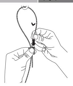
**7.** Press the button on the gripple and slide the safety cable through to the desired height to adjust speaker height.
