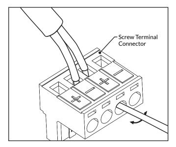
**3.** Connect signal wire to either of the (+) and (-) slots on the screw-terminal connector. Ensure correct polarity and tighten unused terminal screws. Empty slots can be used as speaker loop-outs.
