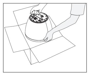
1. Unpack speaker and hanging hardware. Remove the speaker cap to access the stow away handle for easy handling and transporting of the speaker.
