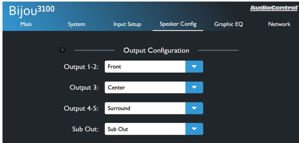
**Output Configuration** - Assign speaker channels each set of outputs, or turn the center and subwoofer channels on or off.
