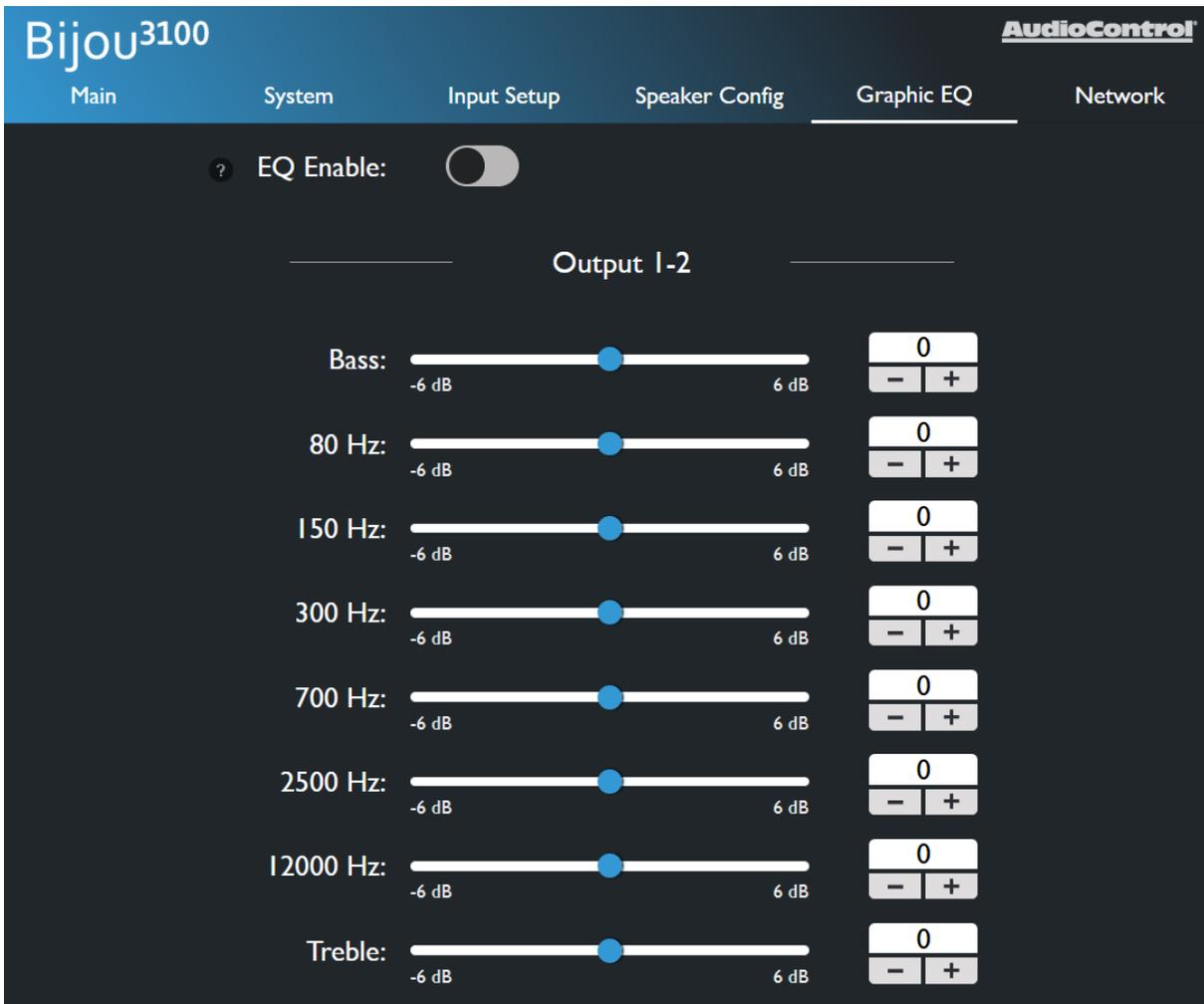
**EQ Enable** - Toggle this ON to apply the EQ curve to the outputs, and turn it OFF to flatten the EQ curve back to default.
