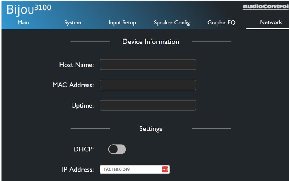
**Device Information** - This section tells you the unit’s Host Name, its MAC Address, and its Uptime (how long it has been powered on).
