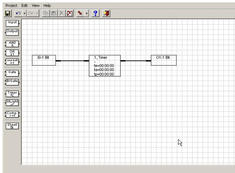
Fig. 87: Delay switch on
