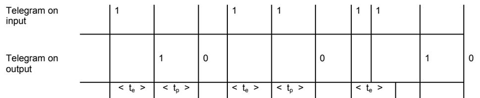
Fig. 96: Diagram "Switch on delay and pulse duration"
