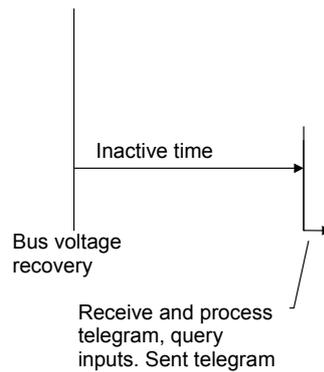
Fig. 21: Behaviour after voltage recovery
