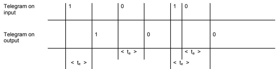
Fig. 92: Diagram "Delay switch on and off"
