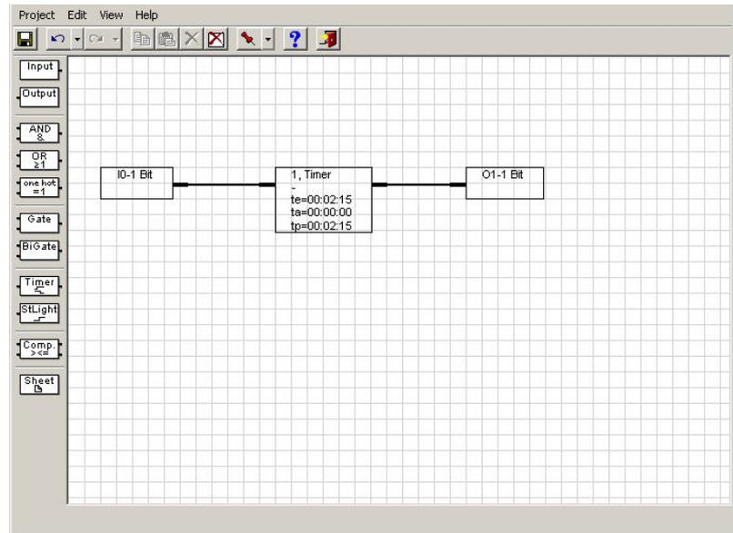
Fig. 95: Switch on delay and pulse duration
