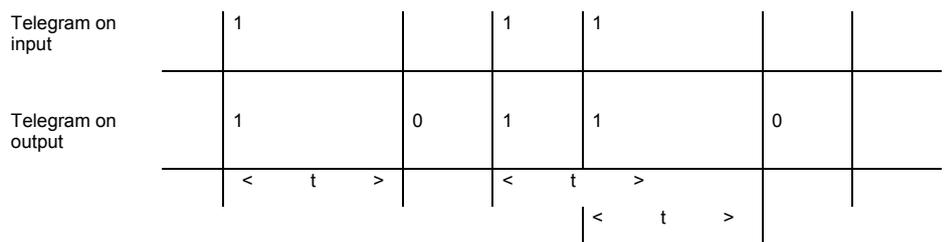
Fig. 99: Diagram "Staircaselight function"
