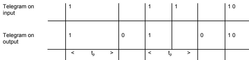
Fig. 94: Diagram "Pulse duration"
