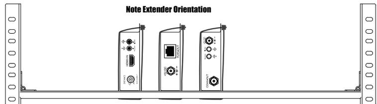
3. Insert one end of the zip tie into the smaller slots from the bottom of the shelf, through the extenders mounting tab, and tighten. Repeat for each extender on the shelf.
