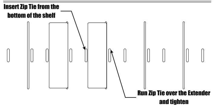
4. Mount the SR-SHELF-MDEXTR in the rack in the desired location. Leave a 1U space below the shelf for easy servicing of the extenders.
