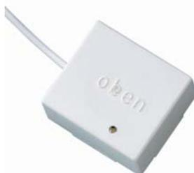
The Water Detector SWM4/RN is used to detect water ingress, e.g. pipe fractures, seepage of groundwater and sewage. The water detector senses rising water via 4 electrodes which are located approx. 1 mm away from the edge of the housing.
