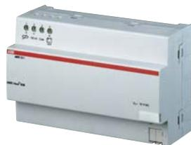
The sealed lead acid battery module AM/S 12.1 is used for maintaining the KNX system voltage and the 12 V DC supply voltage during mains voltage failures. The battery module can only be used in combination with the Uninterruptible KNX Power Supply SU/S 30.640.1 or the Uninterruptible Power Supply NTU/S 12.2000.1.
