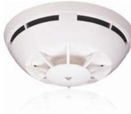
The FC600 fire detector series are conventional threshold alarm detectors that comply to the respective standard of the EN 54 standard series and are VdS approved. The detectors feature an alarm indicator on the detector head that is visible from all angles, and which can be triggered with a permanent magnet for test purposes. A detector base is provided for mounting and cable connection purposes, into which the detector is simply screwed in via the bayonet connection.
