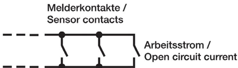
On the other hand, open circuit types are open in the normal state. Should at least one contact close, the circuit is closed and it is evaluated by the Security Terminal.
