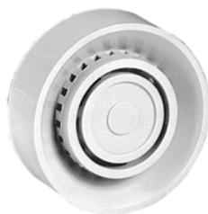
The Electronic Solid-State Siren SSS is used for issuing acoustic alarms within the protected area. An intermittent signal of 2.7 kHz is produced by an electronic tone generator and converted into sound waves by a piezo element.
