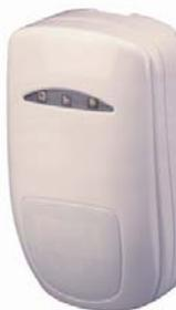
The Passive Infrared Detector IR/K is an intrusion detector (VdS class B) that detects and signals motion within its detection range. It facilitates monitoring of an area with a volumetric IR range of up to 15 m and can be optionally set for hall monitoring function up to 15 m.
