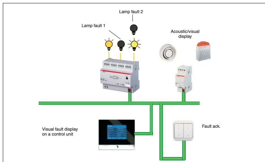
Fig. 31: System representation of a fault signal
