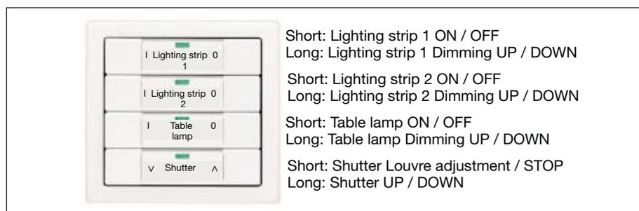
Fig. 33: Push button assignment for “Individual solution”
