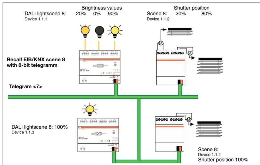
Fig. 27: 8-bit-scene example: Recall scene no. 8
