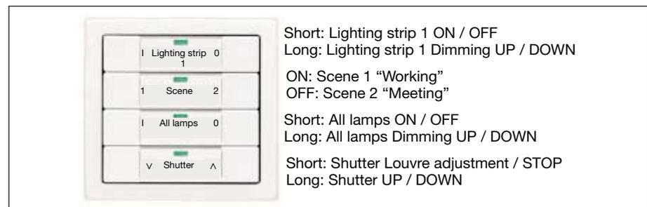
Fig. 34: Push button assignment for “Scene solution”
