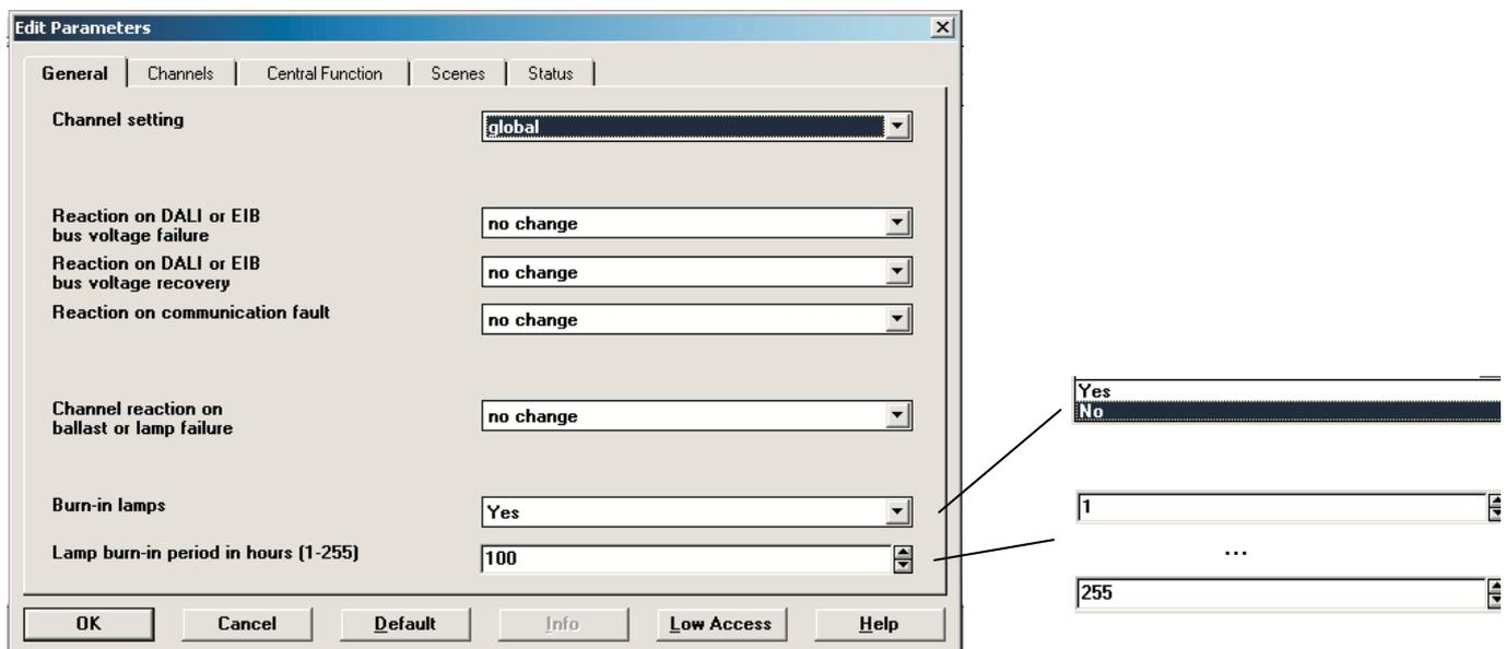
Fig. 19: General parameter window - Burn-in time of lamps
