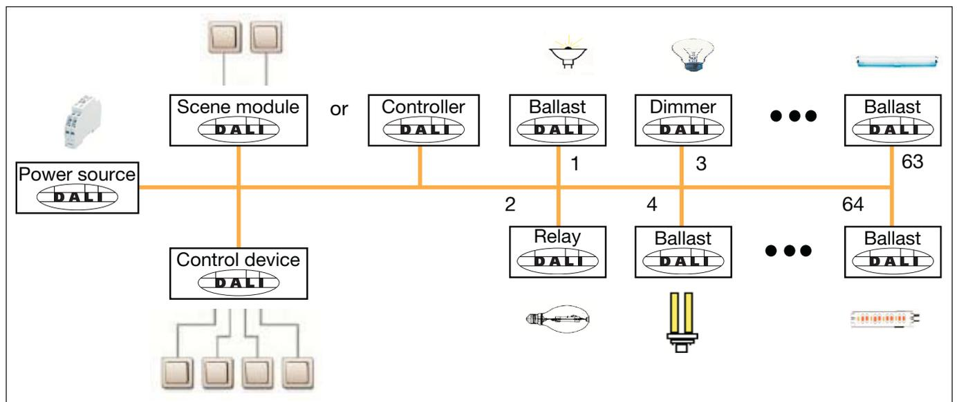
Fig. 2: DALI block diagram
