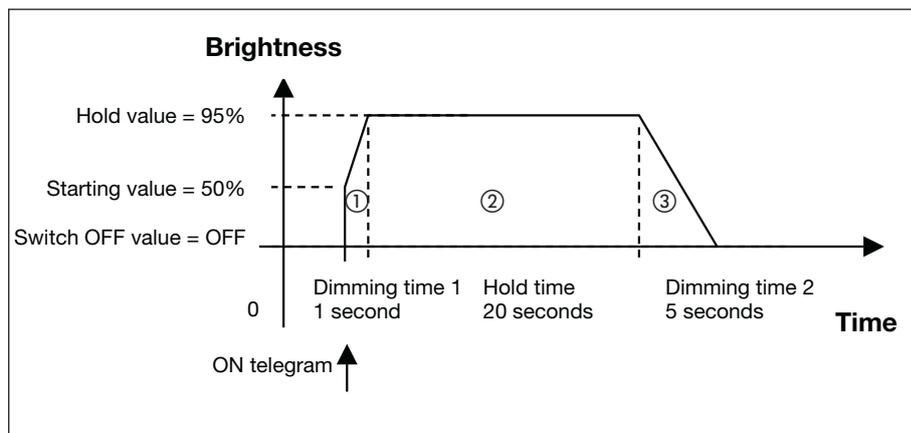
Fig. 30: Timed progression of the staircase lighting function
