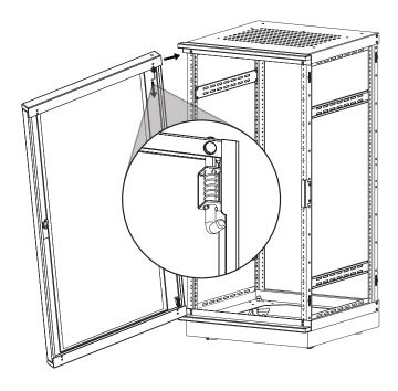
Note: Before installing the door, position the hinge bushings in the holes on the top and bottom brackets on the side that will swing.
