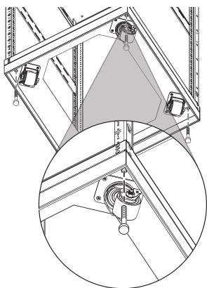
Note: Installing the leveling feet will restrict steering rotation of the casters. If the feet will be used, position the rack before installing equipment.
