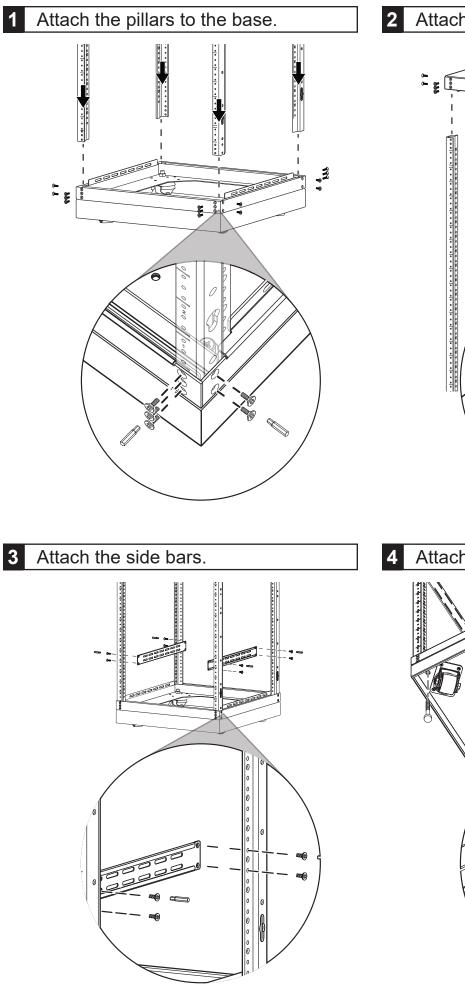
Note: The side bars are not required for structural support and can be mounted at any height. (Two of four included bars are pictured.)
