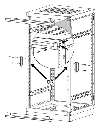
Note: The door may be installed for left or right-hand swing. Hinge brackets are held on by 2 of the 3 assembly screws at each corner.
