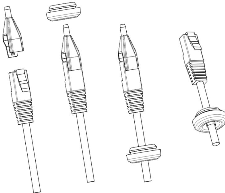
5. Plug the various cables into the appropriate ports on the base of the camera.
