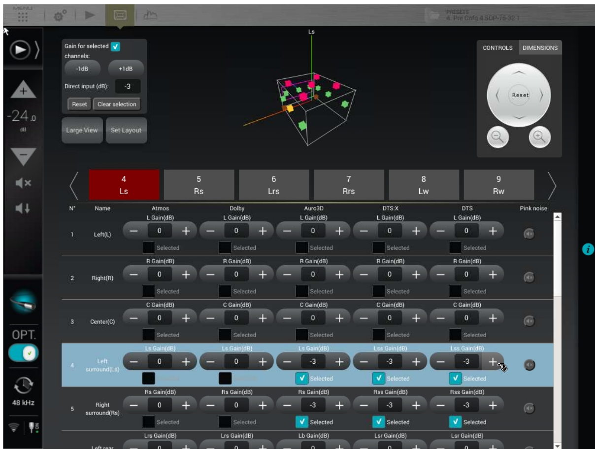
Figure 66: Set gain control panel
