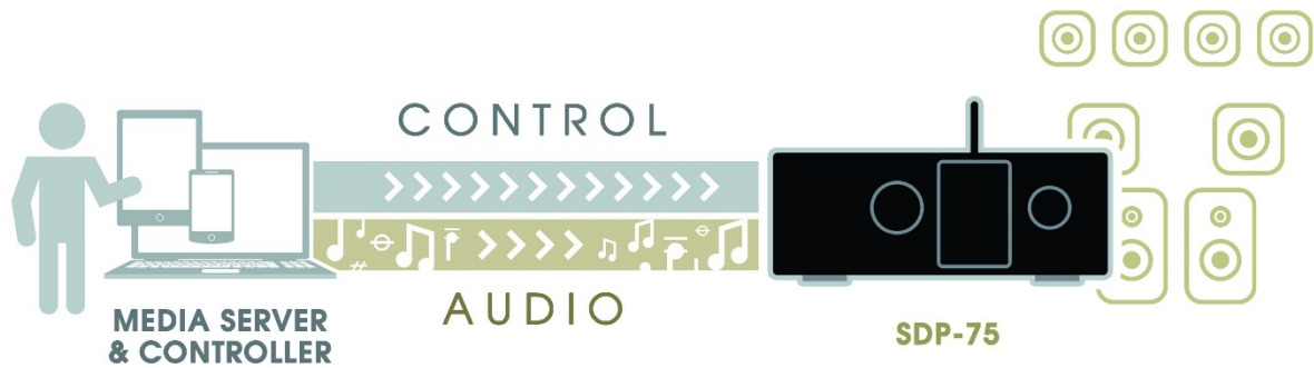
UPnP Network with a device used as server and controller
