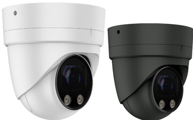
The 8MP Performance Series Turret Camera features a 4K Sony® Starvis™ sensor and includes a 2.7-13.5 mm motorized varifocal lens with autofocus. The camera supports IR night vision up to 25 meters, micro SD card support for local storage up to 512 GB, and features an IP67 rated housing to protect the camera from outside elements.
