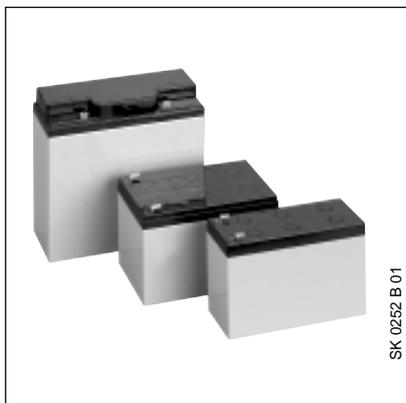
The sealed lead acid batteries SAK7, SAK12 and SAK17 are used to buffer the EIB system voltage in combination with the Uninterruptible EIB Power Supply. A maximum of two sealed lead acid batteries can be connected in parallel to the Uninterruptible EIB Power Supply. In this case, two identical sealed lead acid batteries must be used.
