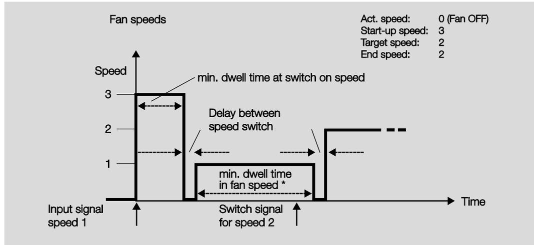
\* The parameter *Minimum dwell period in fan speed in s [0...65,535]* in the parameter window *Automatic operation* is only active and programmable, if the option *yes* has been selected in the *Enable automatic operation* parameter. In the parameter window *Fan*, you can find the parameter *Enable automatic operation*.
