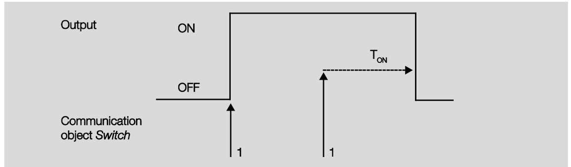
The response is the fundamental response of the staircase lighting function.
