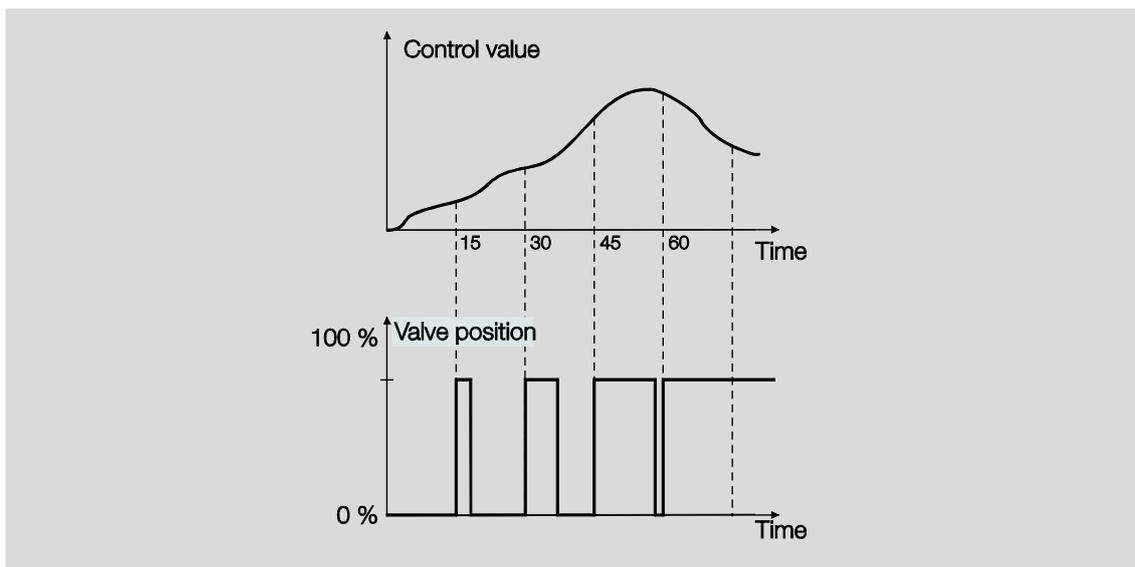
With pulse width modulation, a relatively accurate control of the temperature can be achieved without any resulting overshoots. Simple, attractively-priced control valves can be used. The positioning frequency of the control valve is relatively high.
