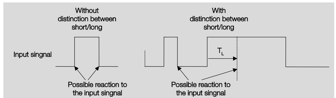
$T_L$  is the time duration from where a long operation is detected.
