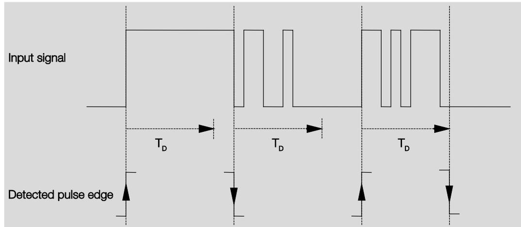
After detection of an edge on the input, further edges are ignored for the debounce time  $T_D$ .
