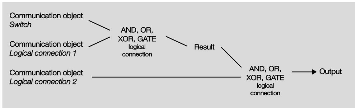
At first the communication object *Switch* is evaluated with the communication object *Logical connection 1*. The result is logically linked with the communication object *Logical connection 2*.
