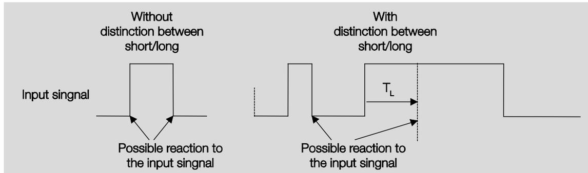
$T_L$  is the time duration from where a long operation is detected.
