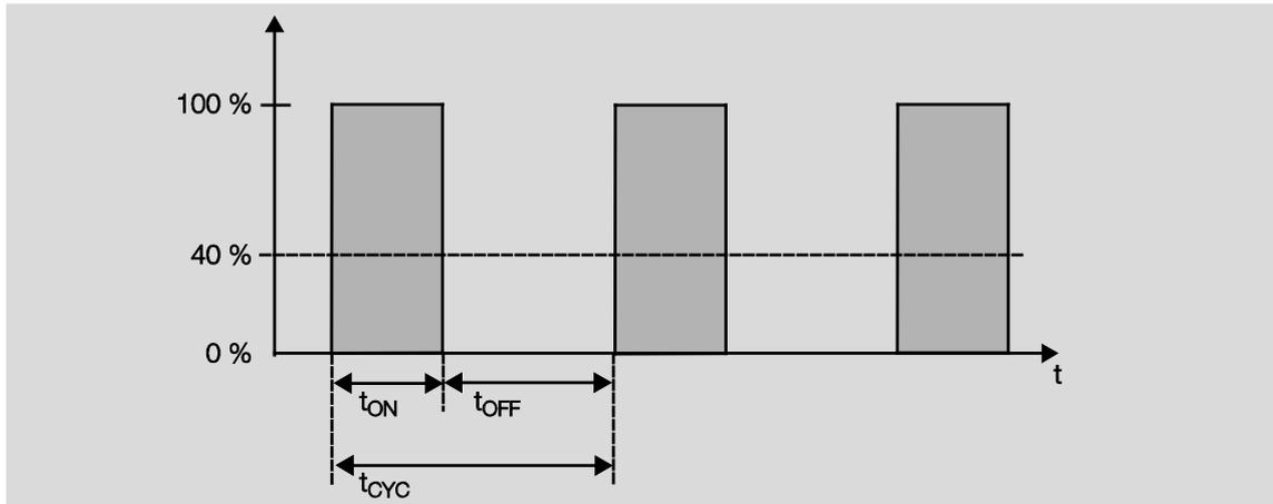
During the time  $t_{ON}$  the valve is opened and during the time  $t_{OFF}$  it is closed.
