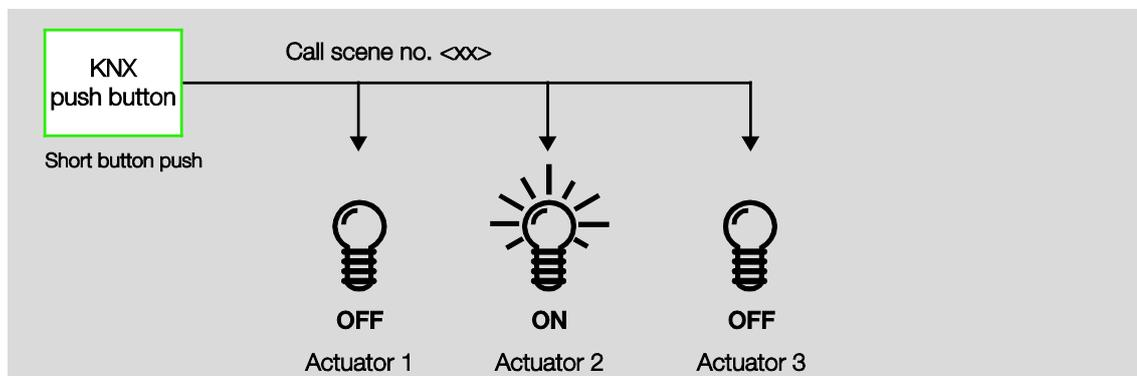
A scene number is sent with the telegram value which must correspond with the scene number in the parameters of the Room Master.
