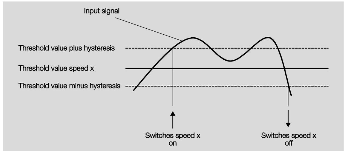
Using hysteresis, a continuous switching between the fan speeds around the threshold value with deviating input signals can be avoided.
