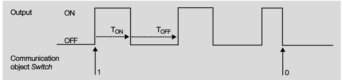
The switch on time ( $T_{ON}$ ) and switch off time ( $T_{OFF}$ ) during flashing can be programmed.
