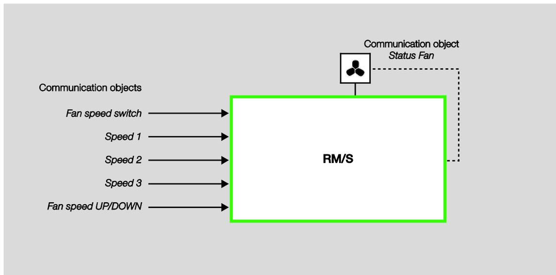
With the three communication objects *Fan speed x switch* ( $x = 1, 2, \text{ or } 3$ ) that are independent of each other, the fan stages are controlled via the outputs of the Room Master.
