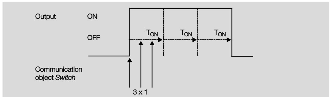
If the device receives a further ON telegram when the staircase lighting is switched on, the staircase lighting time is added to the remaining period.
