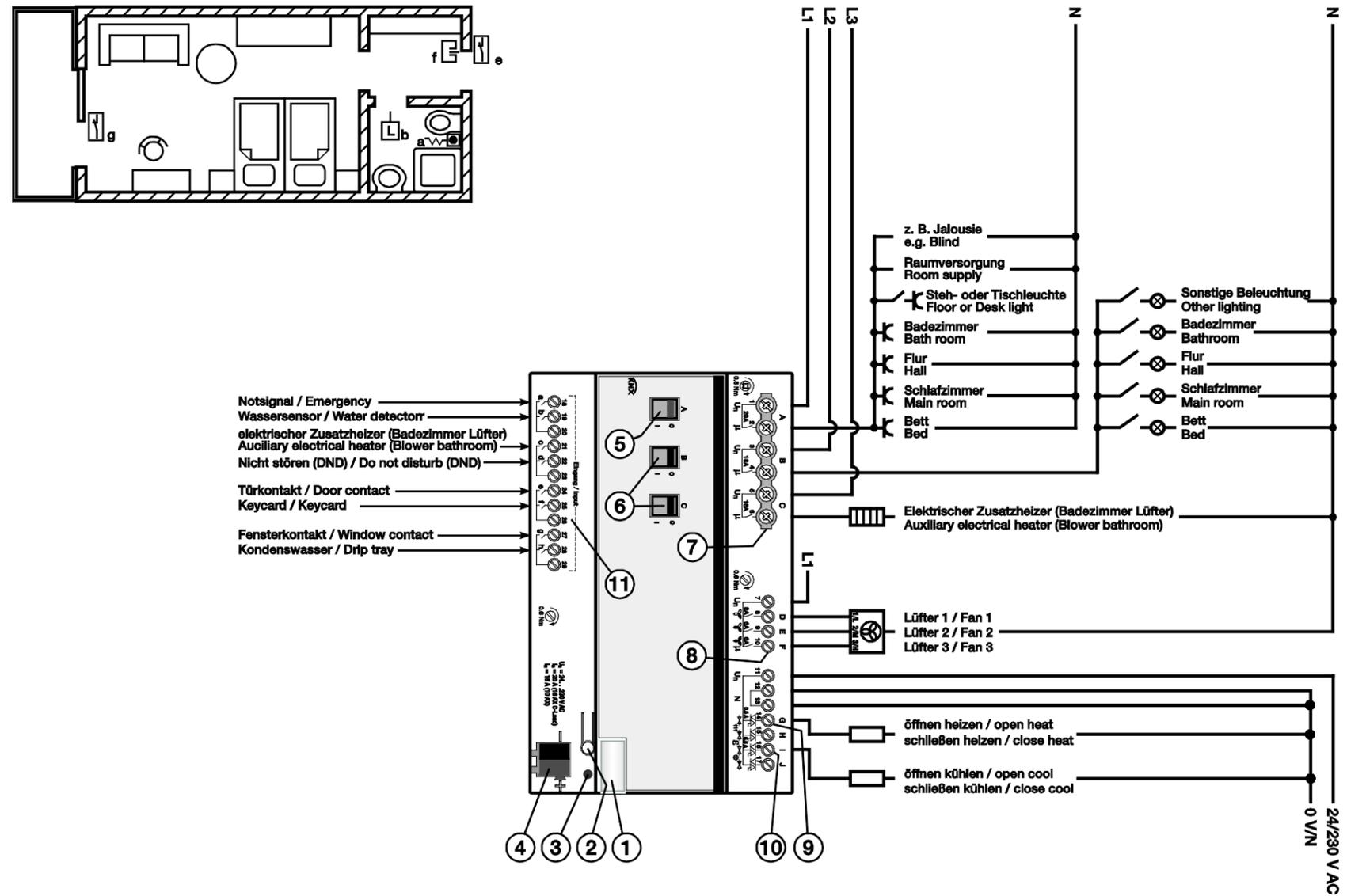
**RM/S 1.1 with electro-thermal valve drives**
