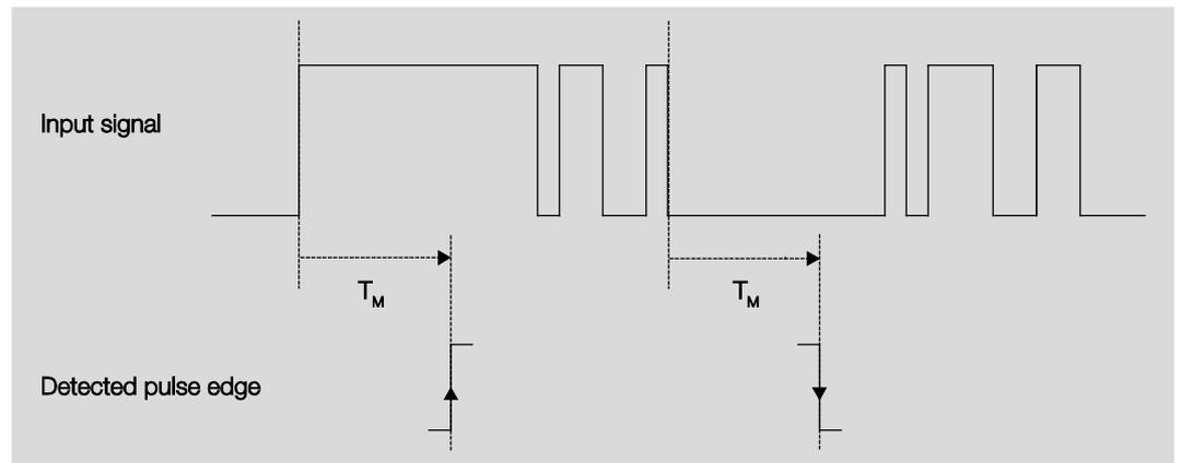
In only two cases, no further edge changes occur within the minimum signal duration  $T_M$  after a change of edge. For this reason, only both of these are detected as valid.
