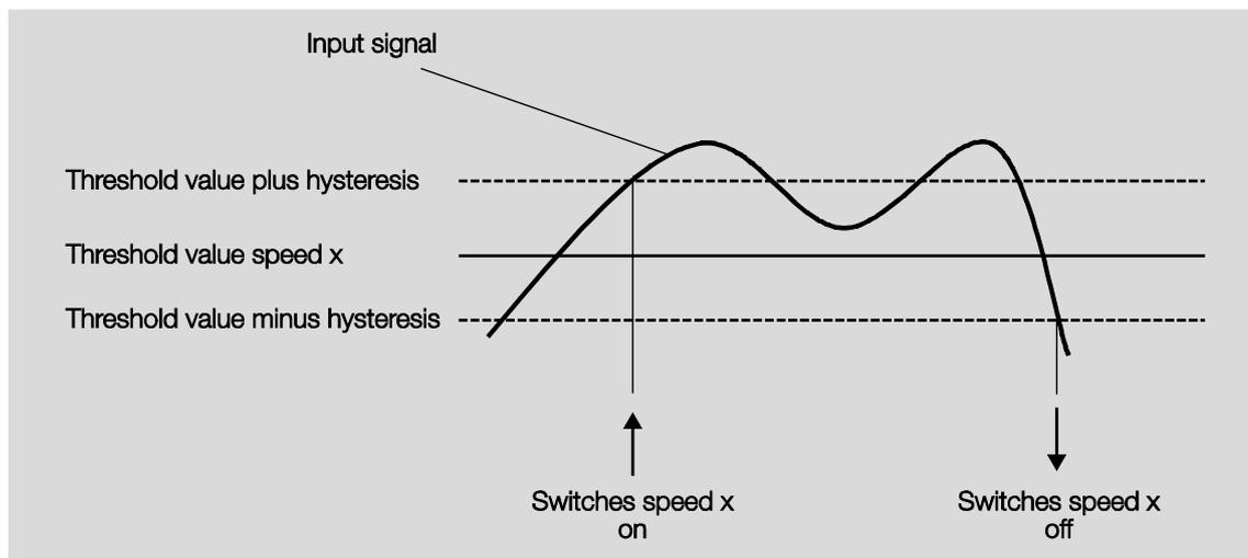
Using hysteresis, a continuous switching between the fan speeds around the threshold value with deviating input signals can be avoided.
