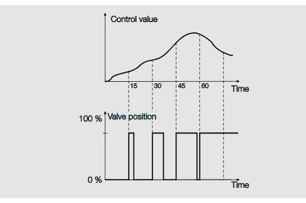
With pulse width modulation, a relatively accurate control of the temperature can be achieved without any resulting overshoots. Simple, attractively-priced control valves can be used. The positioning frequency of the control valve is relatively high.
