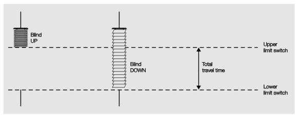
The blind is moved in this direction until the Room Master receives a STOP telegram or the upper or lower limit positions are reached and the motor is switched off by the end limit switch.
