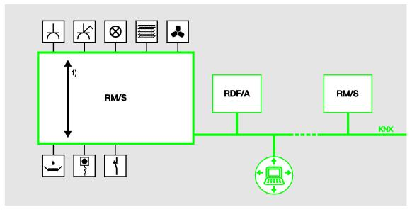
The standard functions of the Room Master are comprised of eight preconfigured room states. All standard functions are activated immediately after the Room Master is connected:
