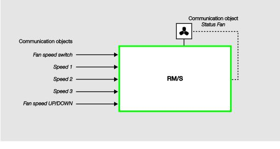
With the three communication objects Fan speed x switch (x = 1, 2, or 3) that are independent of each other, the fan stages are controlled via the outputs of the Room Master.
