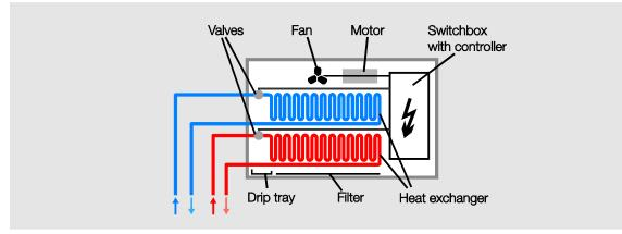
The fan blows air past the heat exchanger and into the room through a filter. The air is heated or cooled in the heat exchangers and thus generates the desired room temperature. The fan is driven by a motor. The motor and the valves are controlled by a Room Master.
