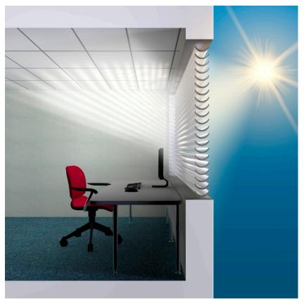
When using special directional slats, the direct daylight into the room is guided, so that the no disruptive direct light penetrates the room but at the same time optimum use is made of the existing natural light.
