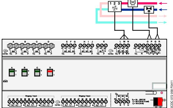
Even the offset of the set point value as well as changeover of the operating modes is implemented by the thermostat. The sensors can be connected directly to the Room Master in order to consider the monitoring of the condensed water and the window contact.
