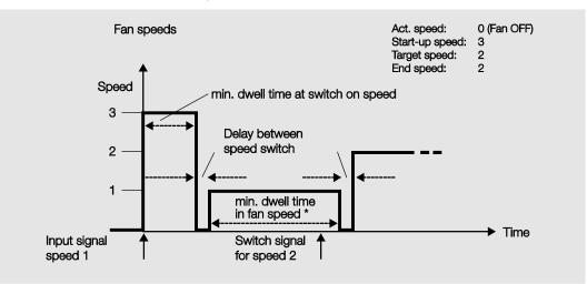
\* The parameter *Minimum dwell period in fan speed in s [0...65,535]* in the parameter window *Automatic operation* is only active and programmable, if the option yes has been selected in the *Enable automatic operation* parameter. In the parameter window *Fan*, you can find the parameter *Enable automatic operation*.
