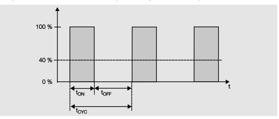
During the time  $t_{ON}$  the valve is opened and during the time  $t_{OFF}$  it is closed. Due to  $t_{ON} = 0.4 \text{ x } t_{CYC}$  the valve is set to about 40 % on.  $t_{CYC}$  is the so-called PWM cycle time for continuous control.
