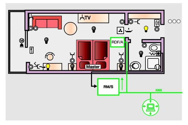
All lights are switched off directly via the outputs with delayed event 2, after the delay time has timed out. Different binary inputs as well as the outlets and the fan in the bathroom are blocked. The displays *Do not disturb, Room occupied, Please wait* as well as *Room service* are switched off. The thermostat, e.g. RDF/A receives a telegram via the bus to change to *Building Protection*.
