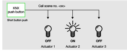
A scene number is sent with the telegram value which must correspond with the scene number in the parameters of the Room Master.
