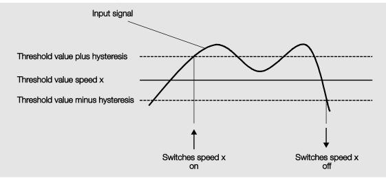
Using hysteresis, a continuous switching between the fan speeds around the threshold value with deviating input signals can be avoided.
