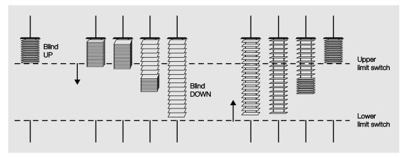
Short movement action can be undertaken by the Room Master in order to purposely adjust the slat angle. Thus the blind is moved for a brief programmed time – the so-called *duration of slat adjustment* – in the required direction and in this way undertakes a slat adjustment (STEP telegram). The smaller the *duration of slat adjustment* selected, the more accurate the adjustment of the slat angle.
