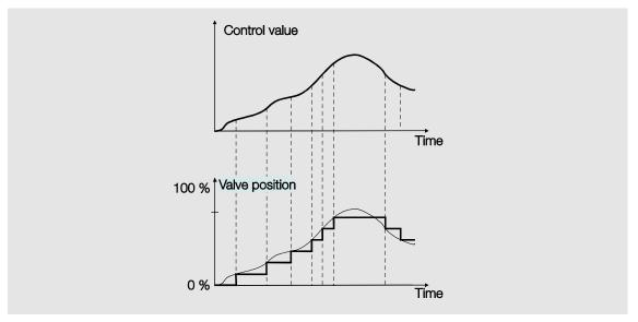
Continuous control is the most precise form of temperature control. At the same time, the positioning frequency of the valve drive can be kept low. Continuous control can be implemented with the Room Master for electro-motor 3-point valve drives. This is implemented via a 1 byte control.
