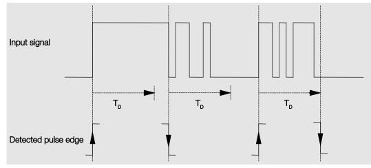
After detection of an edge on the input, further edges are ignored for the debounce time T<sub>D</sub>.
