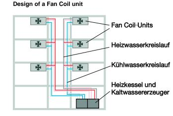
The Fan Coil unit consists of a fan or blower-convector and one or two heat exchangers, which emit heating or cooling power to the room.
