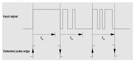
After detection of an edge on the input, further edges are ignored for the debounce time  $T_D$ .
