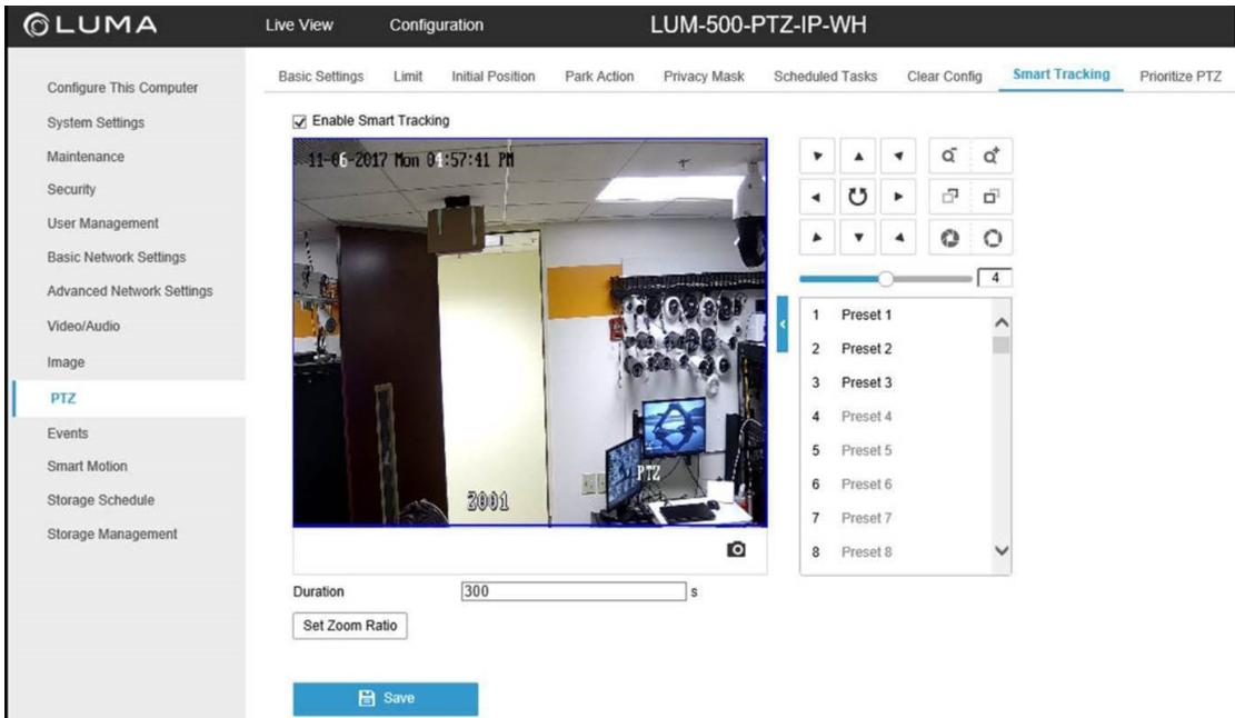
Just above the video screen, click the checkbox to enable smart tracking. Just below the screen, enter the maximum duration of smart tracking (up to 300 seconds). Click **Save**.
