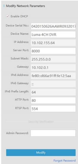
**Suggested Best Practices:** Ensure the **Enable DHCP** box is activated. In your router, reserve an IP address and assign it to the camera's MAC address (found on its box). See your router's documentation for details.
