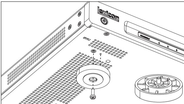
Figure 1. Feet Installation
