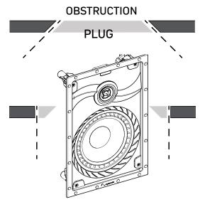
Make a cutout for the speaker using the supplied template. Allow space for the bezel if installing near adjacent objects, or cut the hole in two steps as shown below.
