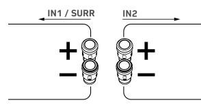
For DVC installs, wire the left channel to either of the two connections and wire the right channel to the other.
