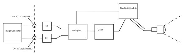
Image 8-55 IG Pixelshift. Principle of operation.
