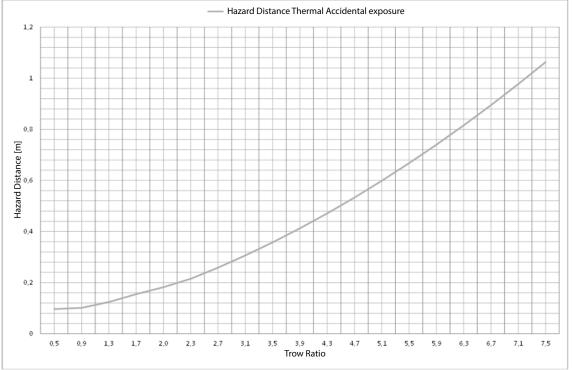
Image 13-5 Hazard Distance in meters versus Throw ratio of the lens for the Balder Cinemascpope projector
