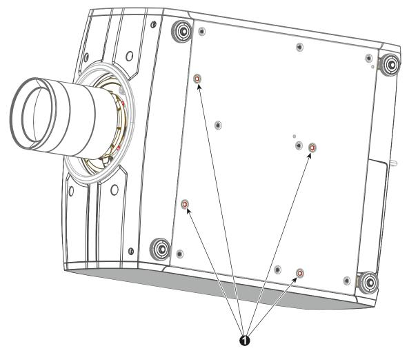
Anchorpoints. For attaching to rigging frame or similar.
