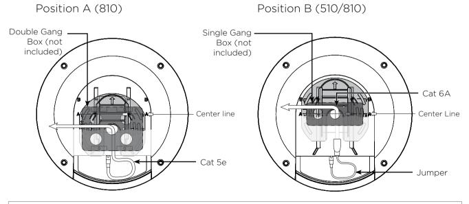
**NOTE:** Jumper is needed when using Cat 6A in Position B.
