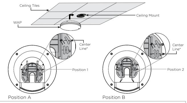
\* Center line of the bracket is not necessarily the center line of the WAP when installed. Please use the guide above to understand the center line of the WAP when installing the bracket.
