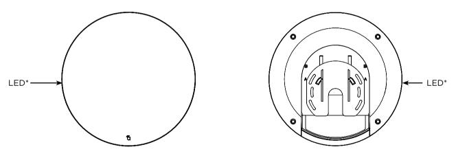
\*NOTE: The LED is located on the side of the device.
