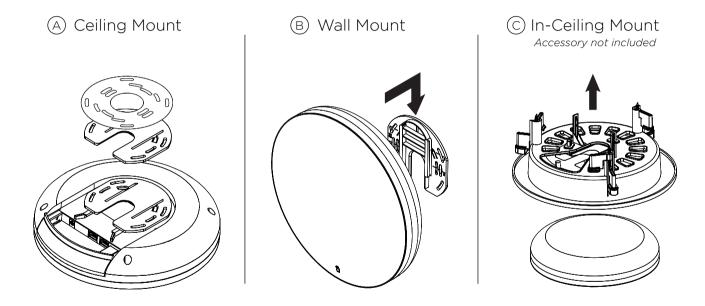
NOTE: Use the ceiling back plate on top of acoustic ceiling tiles to prevent the mounting nuts from pulling through.
